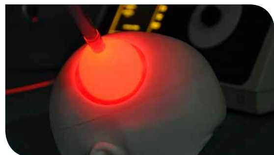
Design of the medical device to deliver PDT during surgery – evaluation of the surgery on a simulation bench
